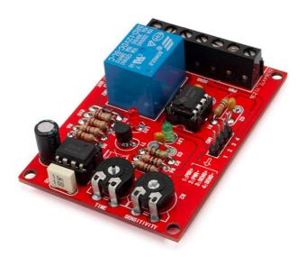
This board, when paired with a rain sensor and connected through a relay, can control the closure of an outdoor blind or a motorized shutter to prevent rainwater from affecting your fixtures. The device features two trimmers that allow you to adjust sensitivity and activation duration.
